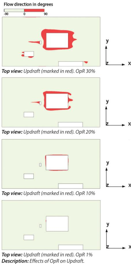
While a 1% OpR eliminates the updraft, the resultant pressure differential is 380 Pa (1.5 in H<sub>2</sub>O). Excessive energy consumption would be incurred to maintain this pressure which would result in very high operating costs.
