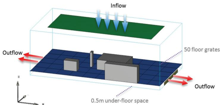
For this example, the computational model consists of a single cleanroom. Some work pieces are placed within the cleanroom that disturb the air flow, but no workers are in the room, and the entrance is not modeled. The inlet and two outlets use fixed flow rates. The raised floor cleanroom uses floor grates, and the entire floor has 50 floor grates.
