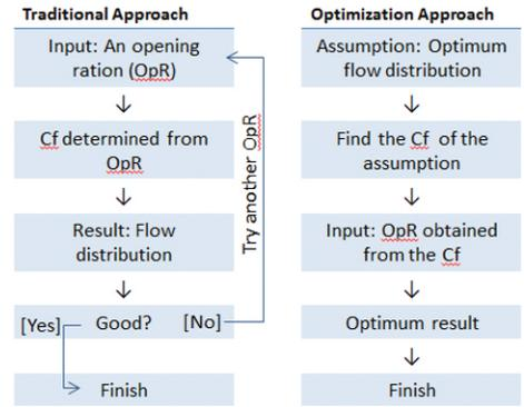
The UDF calculates the pressure loss coefficient through the floor grate (Cf) that will produce the optimum flow distribution. Pressure loss is expressed using the following equation.
