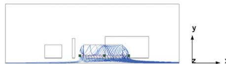
**Section view:** Streamlines near the object. OpR: 10%
