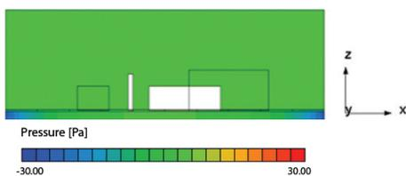
**Section view: y-direction:** Pressure after optimization.
